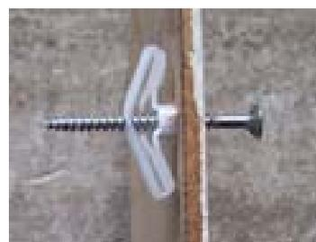
Next comes the hollow wall anchor. Again used individually these are not ideal for fixing heavy objects but as with the toggle above and the spring toggle below, anything that creates a pulling effect from the wall is ideally held at the top with these.
