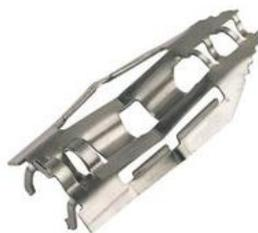
Then we have the Spring (or gravity) toggle or Butterfly fixing. The principle is the same. A hole is drilled, the butterfly wings are held together while the unit is pushed into the hole, the screw is tightened to clamp your fixture to the wall.
